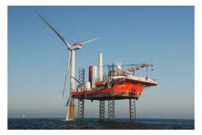
Figure 2.6 Example Construction Vessel (Jackup Barge)
