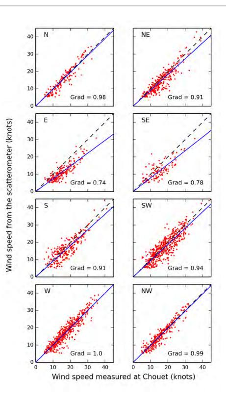
Figure 3 - Scatter plots of winds from Chouet compared to winds from the ASCAT scatterometer, for 8 directional sectors. The 1-1 line is shown as black dashes, and the best fit line (passing through the origin) is shown as a blue line (with the gradient shown).
