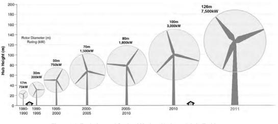
Figure 2.1 Evolution and Scale of Modern Horizontal Axis Turbines (Source: <u>https://commons.wikimedia.org/wiki/File:Wind\_turbine\_size\_increase\_1980-2011.png</u>)
