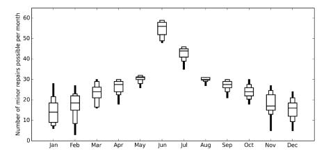
Figure 1 - A 'box and whiskers' plot showing the number of minor repairs that could be carried out by a single workboat operating out of Guernsey. The boxes and whiskers indicate the range of values over the 35 years of simulation. The widest box shows the P25 to P75 percentiles (with a horizontal bar for the median), the narrower box shows out to the P10 and P90, and the narrow 'whisker' shows the most extreme values.
