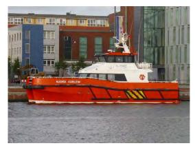
Figure 2.7 Example Crew Transfer Vessel (fast, often multi-hull vessels) (Source: https://commons.wikimedia.org/wiki/File:Ship Njord Curlew.jpg)
