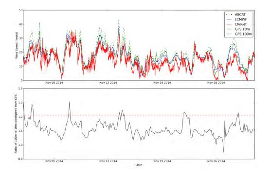
Figure 4 - Wind speed from a range of sources (top), including the US GFS forecasting model at 10m and 100m height (see legend). The bottom plot shows the ratio of 100m wind speed to the 10m wind speed from the US GFS forecasting model – with a constant ratio shown (red dashed line) for comparison (associated with neutral atmospheric conditions over water).
